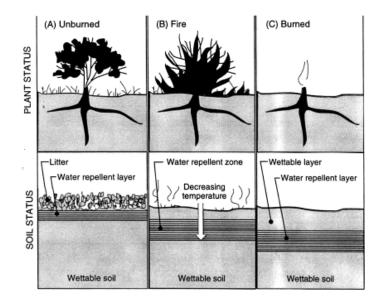
**Fig. 3.** Fire-induced formation/intensification of a water-repellent soil layer (DeBano 2000) Although a fire-induced water-repellent soil layer is said to reduce infiltration, there are instances when an increased infiltration rate was reported after fire (DeBano 1973). This is due to complex relationships between water repellency and soil temperature, as shown in Table 1.
