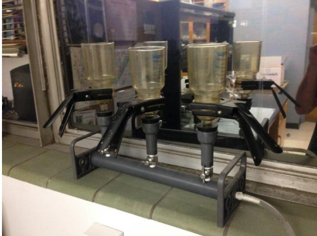
Figure 2: Filtration apparatus used to concentrate phytoplankton from sample water.
