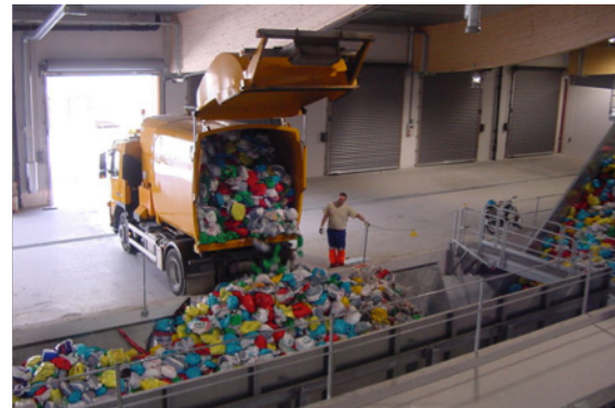
Figure 58: Envac's Optibag optical sorting system.
