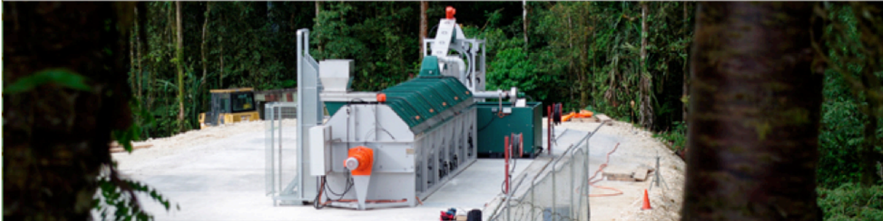
Figure 60: HotRot self-contained composting unit.
