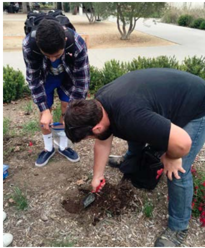
Figure 4. Using a trowel to dig 6 inches into the soil to collect sample.
