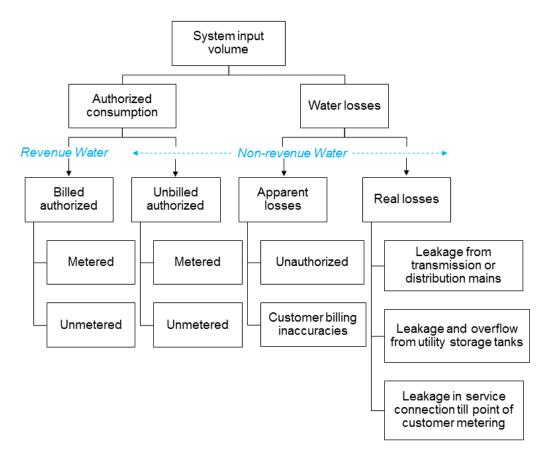
Figure 2 IWA water balance (Lambert A., 2003)
