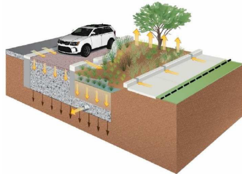
Figure 5-2 Conceptual Schematic of Green Street (arrows indicate water pathways)
