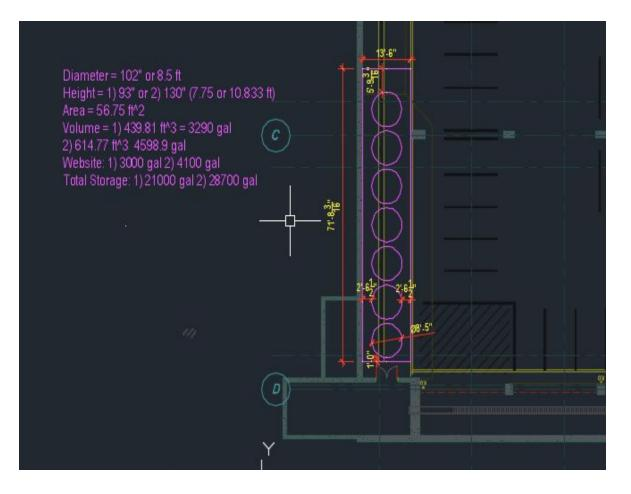
Figure 2a. AutoCad drawings of the cisterns in their proposed location (Parking Structure 9).
