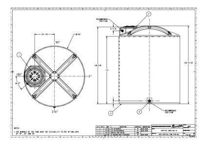
Figure 2b. Cistern measurements.
