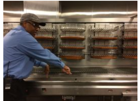
Charles Wilcots pointing towards the trough in which all food waste is poured into.
