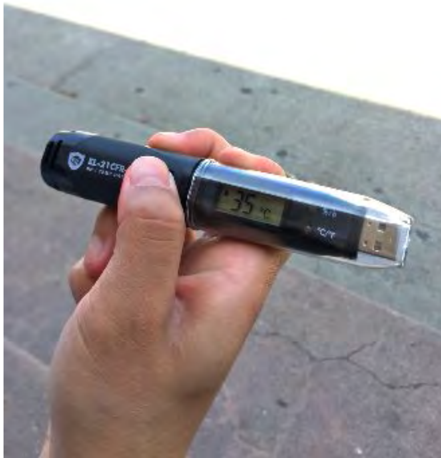
Figure 5: Above is an image of a sensors purchased from Dataq Industries, model number EL-USB-2-LCD. A San Fernando team member is holding it during data collection.
