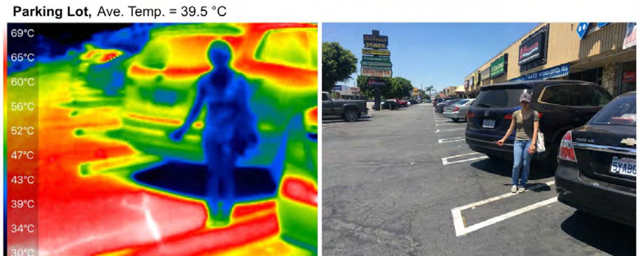
Figure 9: Side-by-side images displaying the unseen heat of asphalt. The hottest point in this frame reaches 69 °C. (Equipment used: Seek Thermal XR Imager for iOS-Apple)
