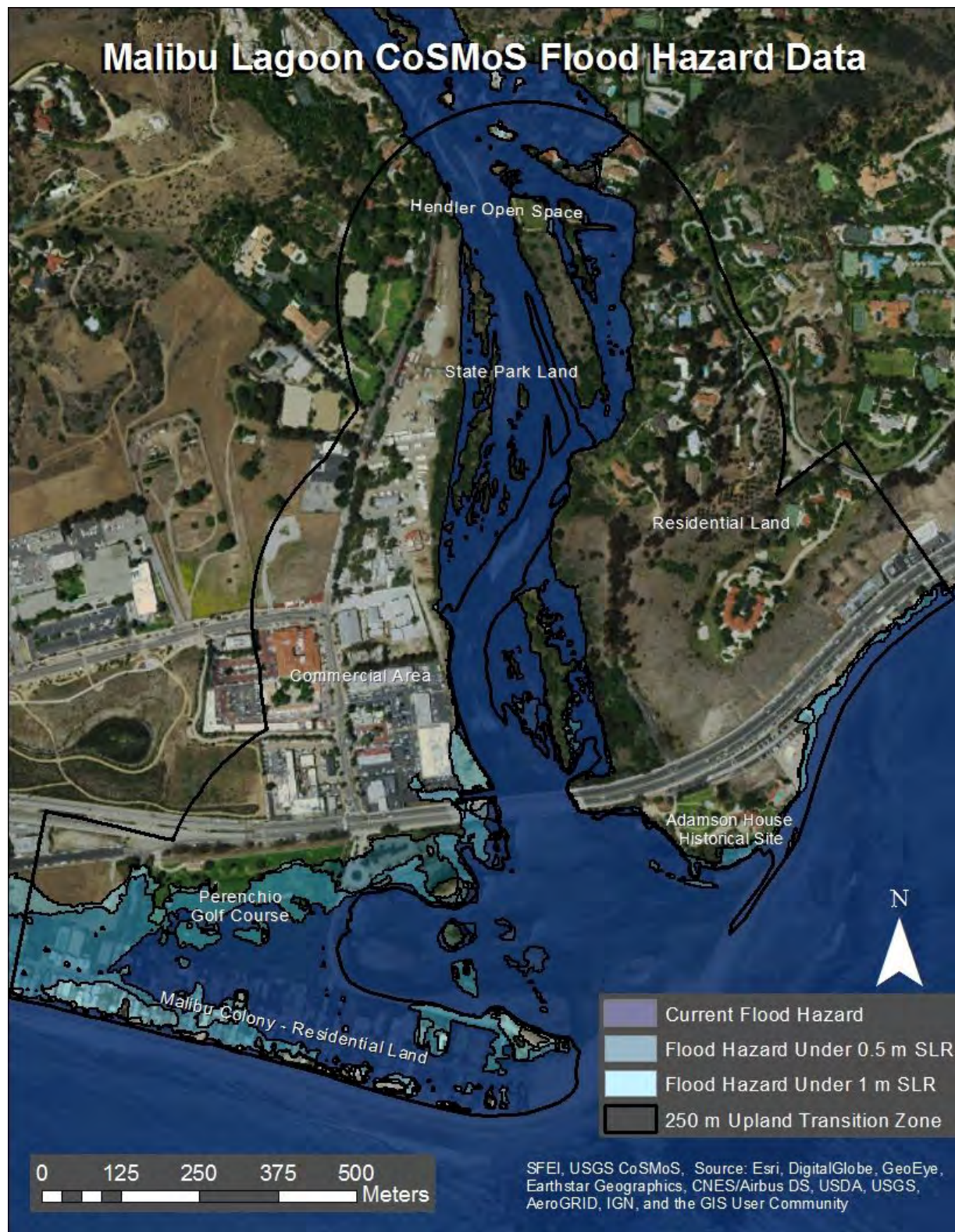
Figure 5: Map of CoSMoS 100-year storm flood risk data under current sea level and predicted sea level changes.
