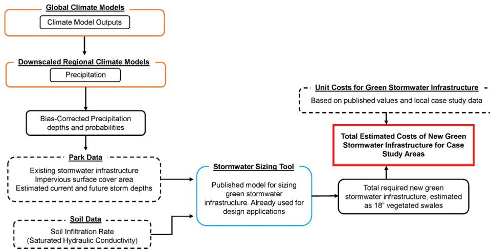
**Figure 1.** Analysis procedures used to apply estimates of downscaled regional climate model outputs to the case study areas.
