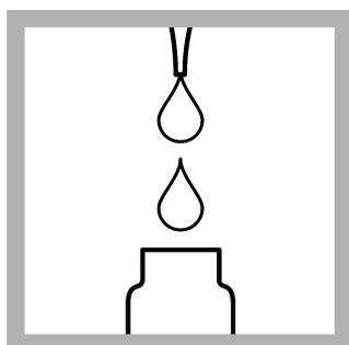
2. Add 5.0 mL of sample to a Reactive Phosphorus Test 'N Tube Vial.
