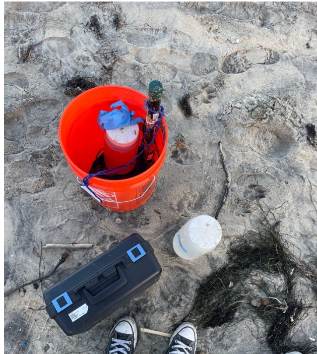
Figure 9: Sampling tools (self-assembled collection bucket, sampling bottles, Turbidimeter™ )
