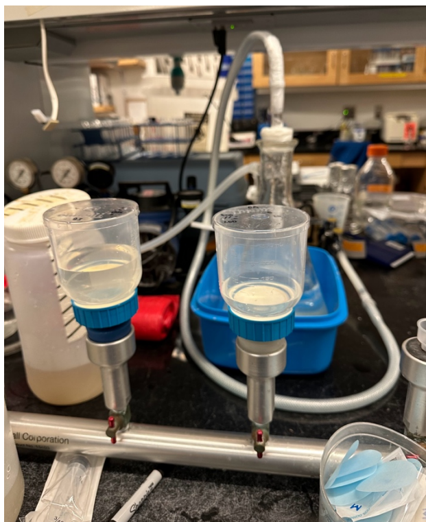
Figure 11: Membrane filtration experiment setting.
