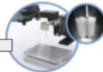
Fig. 1.6. QX200 Droplet Reader autosampler.
