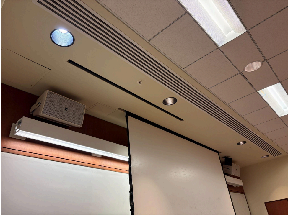
Figure 5. Ceiling Openings for Overlapping Projector Screens in PAB 2434
