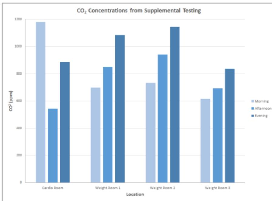
**Figure 6:** This graph shows the concentration of carbon dioxide (CO<sub>2</sub>) during three different time intervals - morning, afternoon, and evening - in four supplemental rooms at the John Wooden Center.
