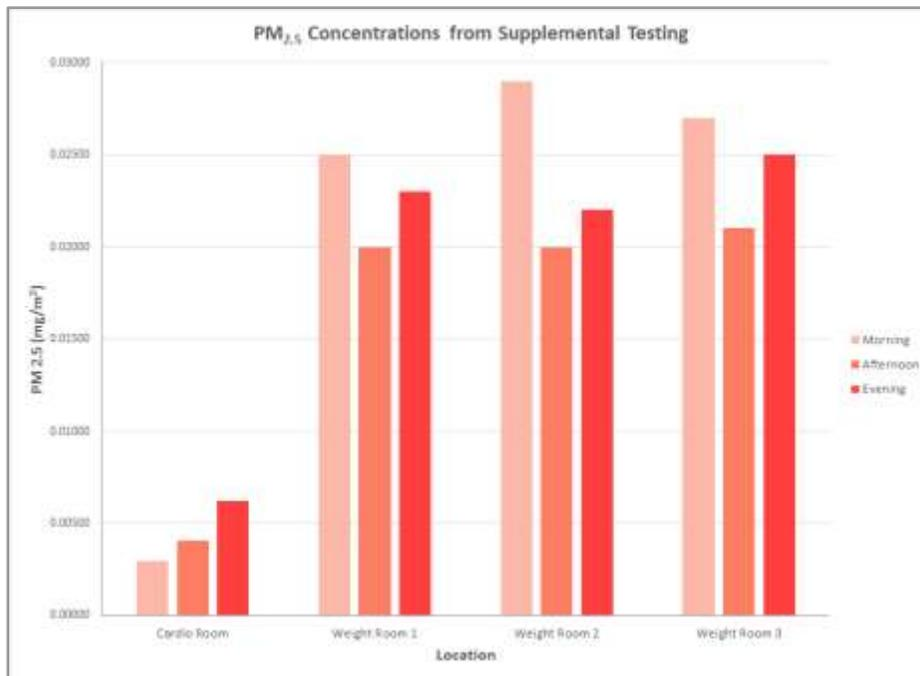
**Figure 9:** This graph shows the concentration of particulate matter (PM 2.5) during three different time intervals - morning, afternoon, and evening - in four supplemental rooms at the John Wooden Center.
