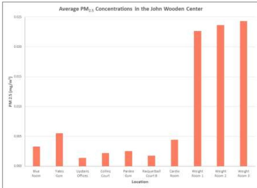
**Figure 7:** This graph shows the average concentration of particulate matter (PM 2.5) in ten different rooms at the John Wooden Center.
