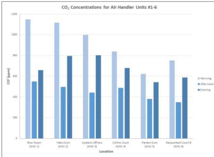
**Figure 5:** This graph shows the concentration of carbon dioxide (CO<sub>2</sub>) during three different time intervals - morning, afternoon, and evening - in rooms according to each of the six Air Handler Units (AHUs) at the John Wooden Center.
