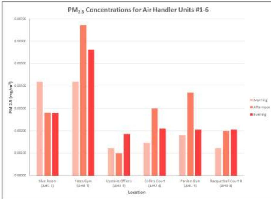
**Figure 8:** This graph shows the concentration of particulate matter (PM 2.5) during three different time intervals - morning, afternoon, and evening - in rooms according to each of the six Air Handler Units (AHUs) at the John Wooden Center.
