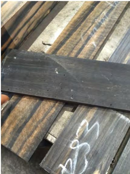
Figure 6. Holes in Ebony Plank
