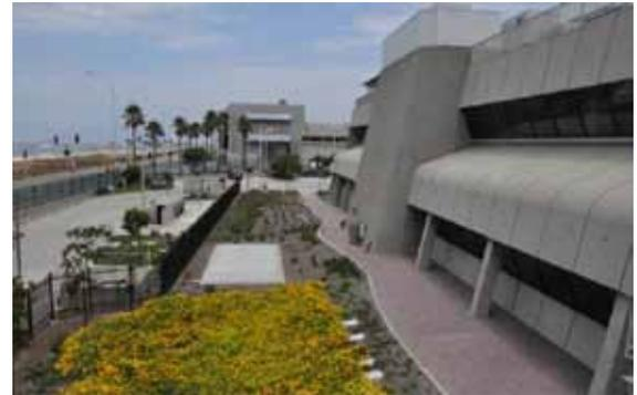
Another outdoor feature of ELC is a bioswale that captures runoff from the building roof drains for percolation. It is lined with native grasses and prevents site runoff and pollution to adjacent areas. The pedestrian bridge above it leads to the beach across the street.
